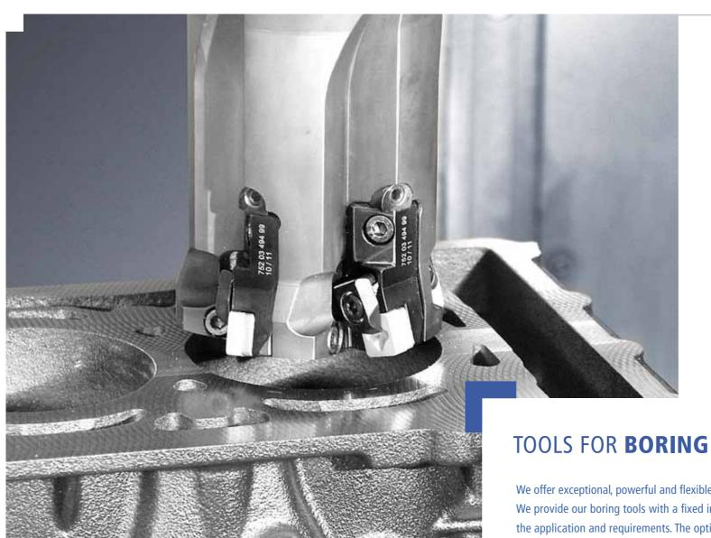
We offer exceptional, powerful and flexible tool solutions for boring applications: We provide our boring tools with a fixed insert seat or cartridge depending on the application and requirements. The optimum number of insert seats ensures that our boring tools are extremely economical. We offer interfaces to all common tool holding systems.
